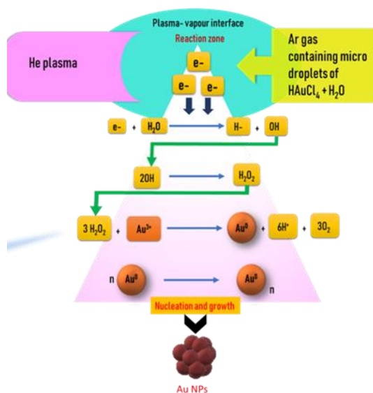
Figure 1. Mechanism of formation of gold nanoparticles inside plasma.
