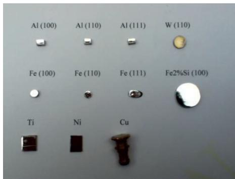
**Figure 4:** Samples used to measure the AES and XPS spectra.
