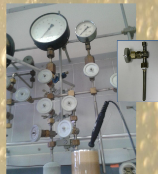
Solubility experiments and reaction vessels used for liquid (left) and near – supercritical (right) xenon.
