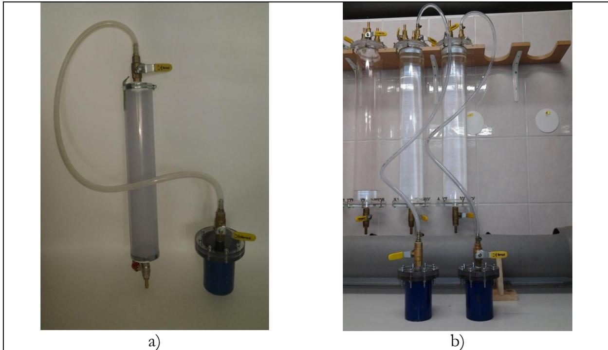
**Figure 2:** Modified equipment for desorption experiments. Lost gas content determination equipment (left), laboratory desorption equipment (right) (Jamnikar, 2011-2012).
