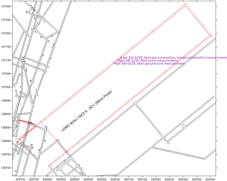
**Figure 6:** Location of seam gas pressure and rock stress measurements at long-wall face K. -50 C (Mine Pesje)
