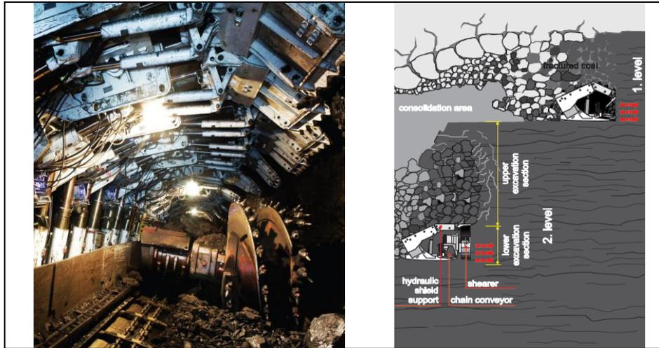
**Figure 1:** Long-wall face with hydraulic steel shield support, shearer and chain conveyor (left) and schematic presentation of lignite seam division into levels, together with sequence of sub-caving excavation in levels (left) (Premogovnik Velenje, 2011)
