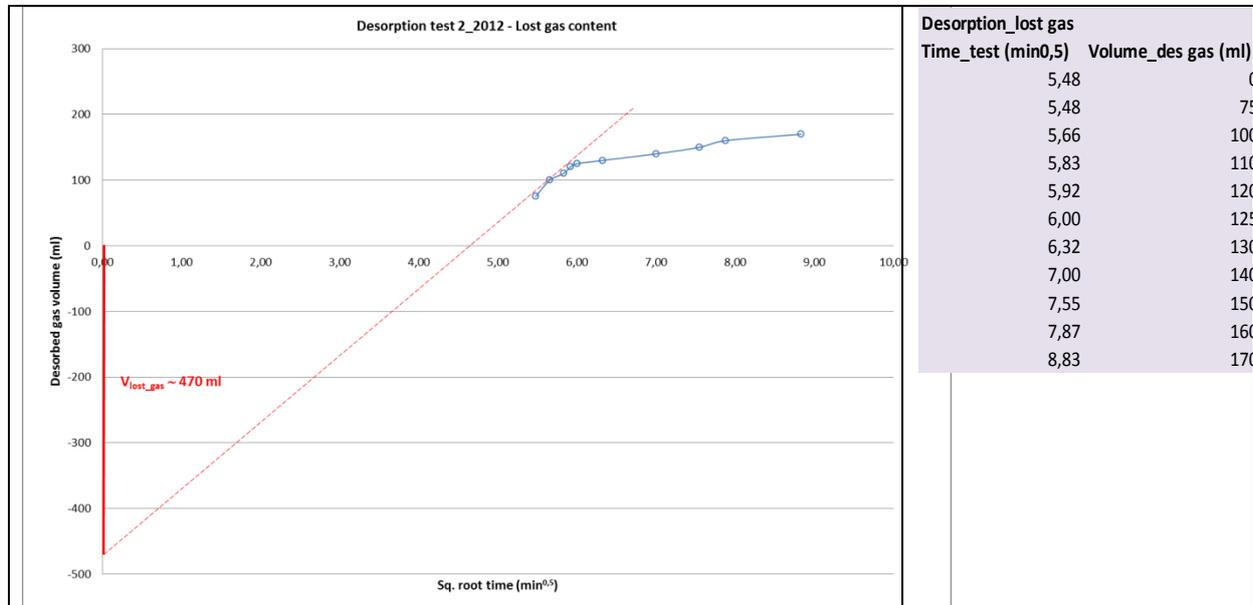
**Figure 3:** Desorption experiment 2/2012 – Lost gas content
