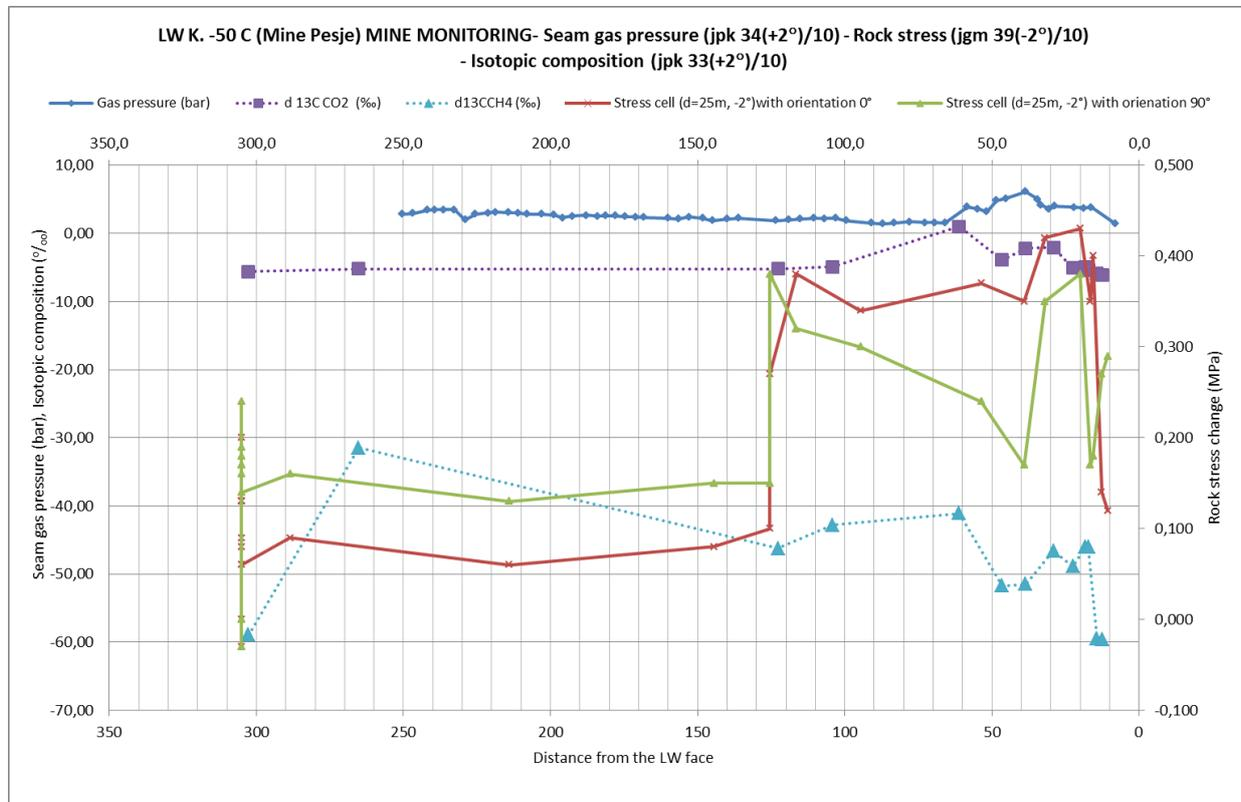
**Figure 7:** Relation between seam gas pressure and rock stress state change in dependence of distance to long-wall face. Rapid increase of stress at distances 305 m and 125 m represent stress cell settings with additional fluid injection.
