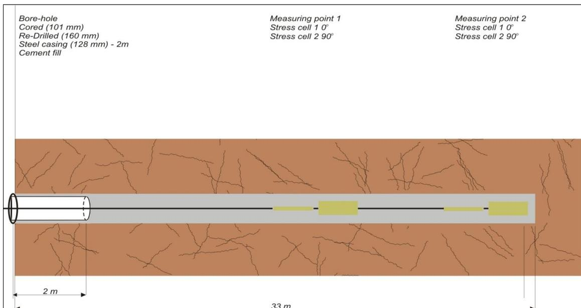
**Figure 2:** Scheme of rock stress monitoring well construction (Jamnikar, 2012)
