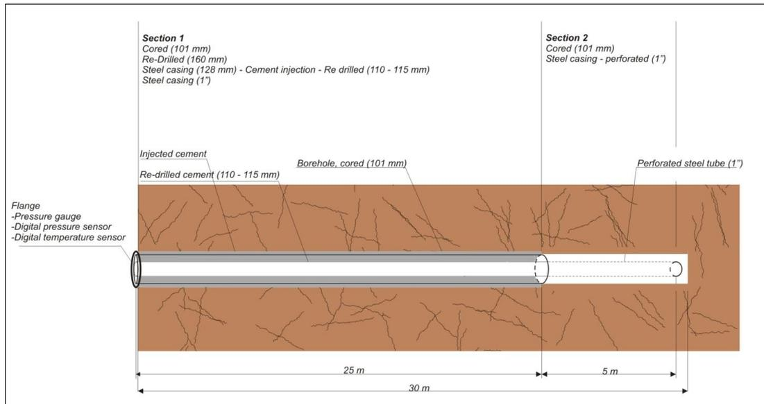
**Figure 4:** Scheme of seam gas monitoring well construction (Jamnikar, 2010)
