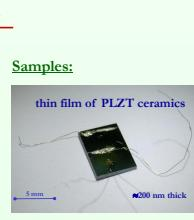
We can conclude that direct measurements confirm existence of the giant electrocaloric effect in thin PLZT films i.e., the PLZT thin films are the best electrocalorics.
