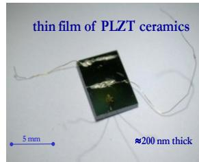
**Figure 3:** Thin film of 8/65/35 PLZT ceramics.
