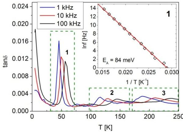
**Figure 4:** Temperature dependence of dielectric losses  $\tan\delta$  of the  $\text{KTaO}_3$  ceramics measured at several frequencies. Different frequency dispersion regions are marked with numbers. The Arrhenius plot from the dispersion region 1 is shown in the inset.  $E_A$ ...activation energy.
