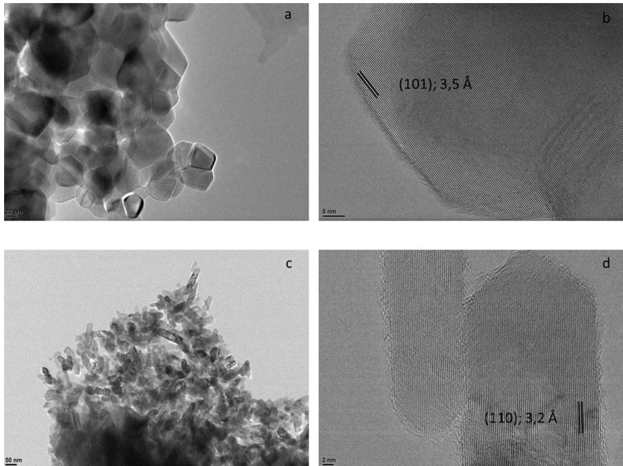
**Figure 1:** TEM images of anatase (a, b) and rutile (c, d) particles prepared by different techniques: (a) and (b) HT\_isopropoxide; (c) and (d) HT\_peroxotitanium.
