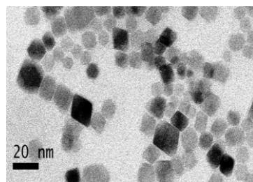
**Figure 4:** TEM image of our magnetic nanoparticles.
