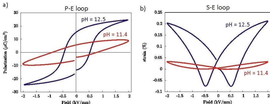
**Figure 5:** Electrical properties of the 0.65PMN-0.35PT ceramics prepared at pH 11.4 (red) and pH 12.5 (blue). a) Polarization vs. electric field. b) Strain vs. electric field.
