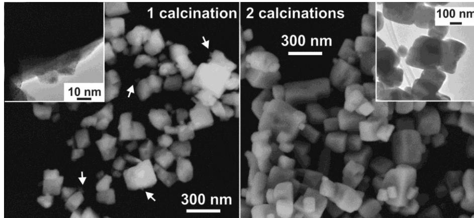
**Figure 1:** FE-SEM micrographs of the powders after one and two calcinations at 800 °C for 4 h. Detailed TEM micrographs are shown in the insets.
