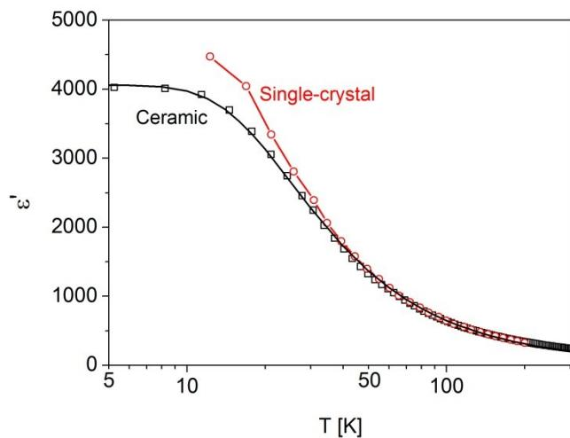
**Figure 3:** Temperature dependence of the dielectric permittivity  $\epsilon'$  of the  $\text{KTaO}_3$  ceramic measured at 100 kHz and single-crystal calculated from the hyper-Rayleigh spectra.[6] The line through the experimental points of the ceramic is fit to the Barret formula, while in the case of the single-crystal it is guide to the eye only.
