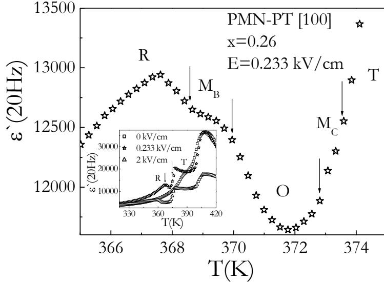
**Figure 1:** Intermediate monoclinic phase sequence observed in the dielectric response of  $\text{PMN}_{0.74}\text{-PT}_{0.26}$  single crystal in [100] direction.
