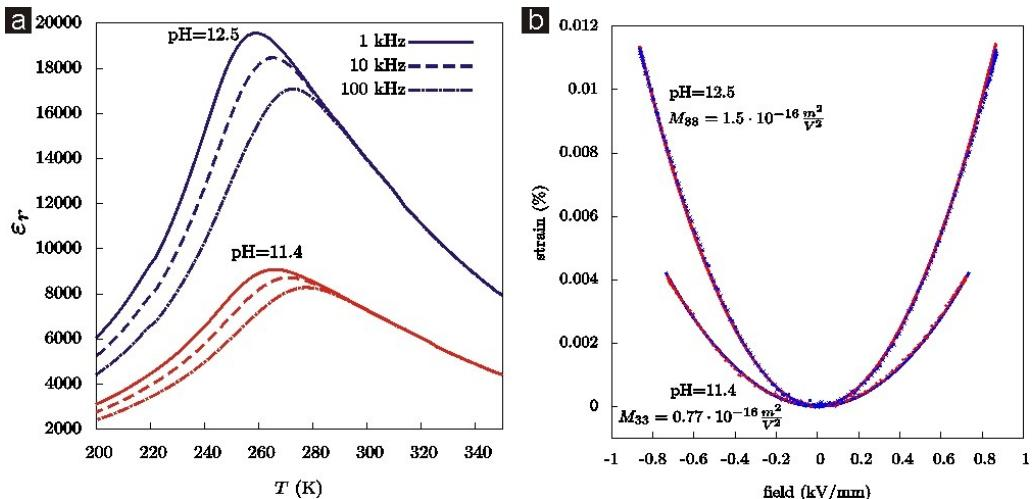
**Figure 4:** Electrical properties of the PMN ceramics prepared at pH 11.4 (red) and pH 12.5 (blue). a) Dielectric constant vs. temperature. b) Electrostrictive properties: strain vs. electric field.
