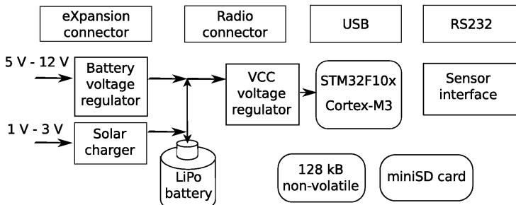
**Figure 1:** Versatile Sensor Node core module block diagram
