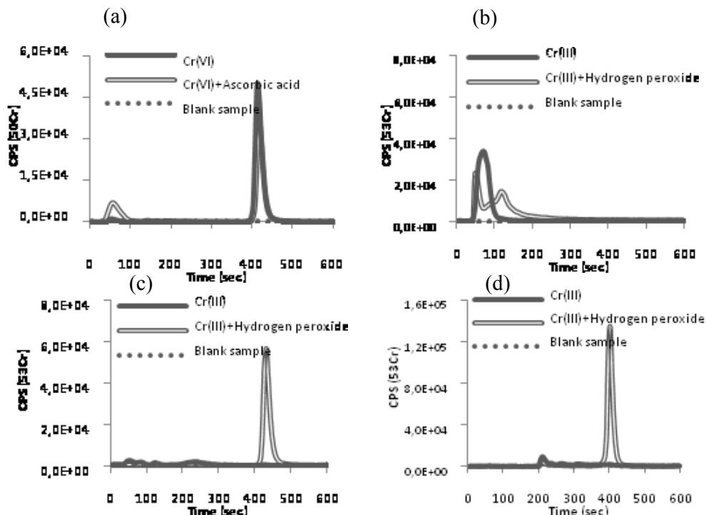
**Figure 2:** The influence of oxidising and reducing agents on speciation of Cr: (a) at pH 4,  $^{50}\text{Cr(VI)}$ +ascorbic acid; (b) at pH 4,  $^{53}\text{Cr(III)}$ +H<sub>2</sub>O<sub>2</sub>; (c) pH 7,  $^{53}\text{Cr(III)}$ +H<sub>2</sub>O<sub>2</sub>; (d) pH 12,  $^{53}\text{Cr(III)}$ +H<sub>2</sub>O<sub>2</sub>
