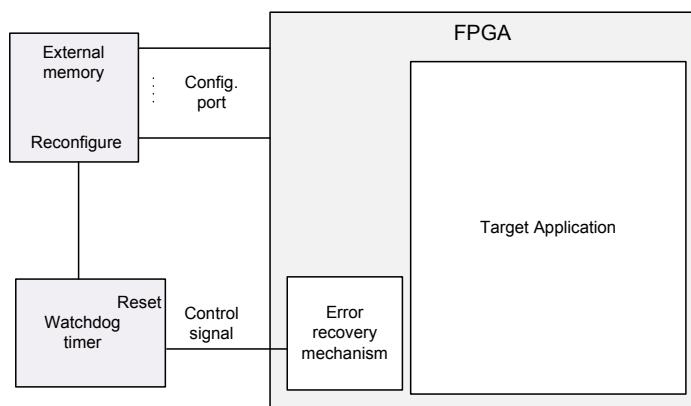
**Figure 3:** Self-reparable system with an external watchdog timer
