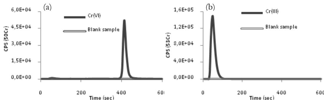
**Figure 1:** (a) Speciation of  $^{50}\text{Cr}$ (VI) ( $10 \text{ ng mL}^{-1}$ , pH 5) and (b)  $^{53}\text{Cr}$ (III) ( $23 \text{ ng mL}^{-1}$ , pH 5) by the FPLC-ICP-MS
