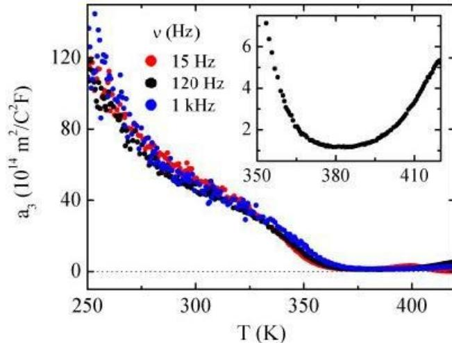
**Figure 2:** Temperature dependence of the dielectric nonlinearity  $a_3$ . Inset shows a paraelectric-to-glass transition in the temperature region where relaxor dynamics dominates the dielectric response.
