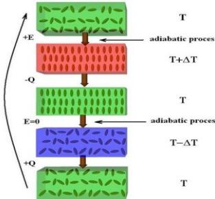
**Figure 2:** Schematic representation of the electrocaloric cycle.
