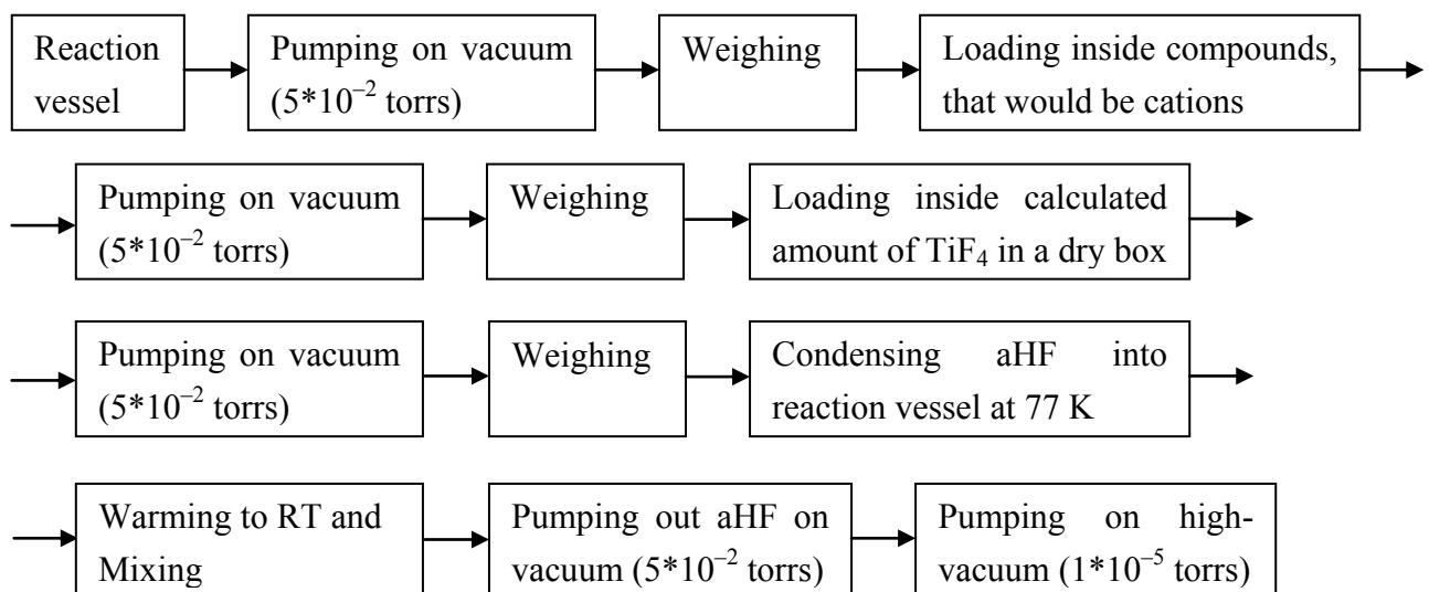
**Figure 2:** The usual procedure of the synthesis
