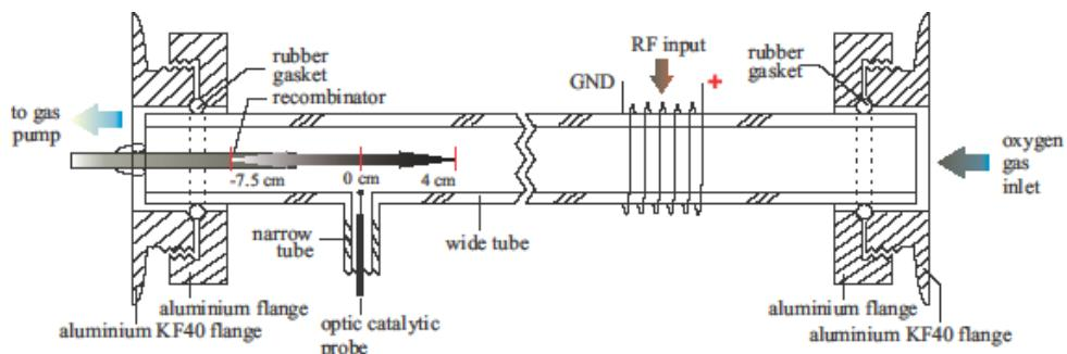
**Figure 1.:** Schematic of plasma system.
