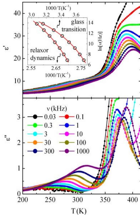
**Figure 1:** Temperature dependence of the real,  $\epsilon'$ , and the imaginary,  $\epsilon''$ , parts of the complex linear dielectric constant. Inset shows the Vogel-Fulcher dependence of the characteristic relaxation times for the relaxor dynamics and glassy transition.
