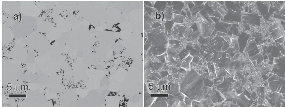
**Figure 2 :** FE-SEM micrographs of the a) polished and b) fractured surfaces of the  $\text{KTaO}_3$  ceramics obtained by back-scattered and secondary electrons imaging modes, respectively.
