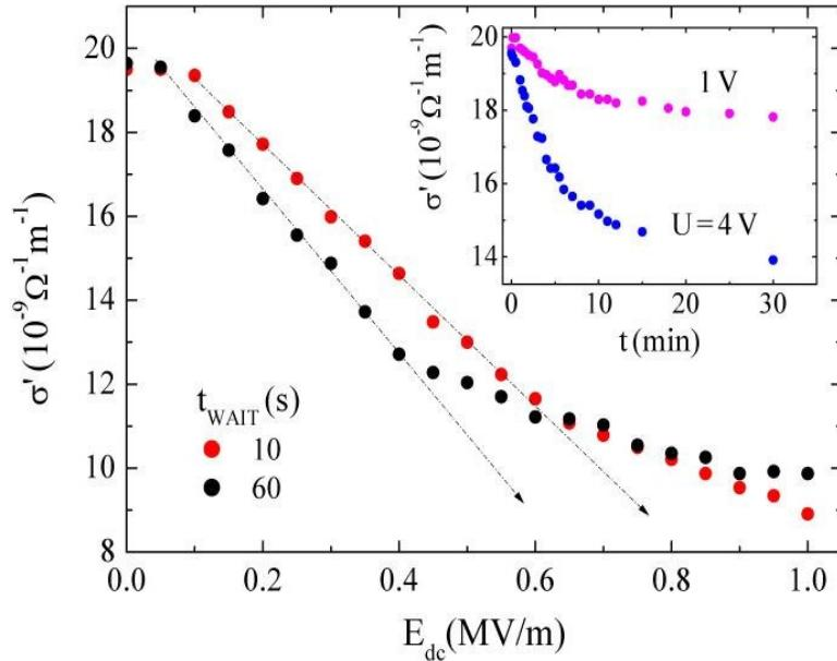
**Figure 4:** The electrical conductivity (at 110 Hz) as a function of the dc bias electric field, detected with two different field change rates - the waiting time between two subsequent points was either 10 s or 60 s. The arrows point towards anticipated ac conductivity blocking field. Inset shows the time-decreasing of the ac conductivity under applied bias voltages of 1 V and 4 V, corresponding to the dc bias fields of 0.05 MV/m and 0.2 MV/m, respectively.
