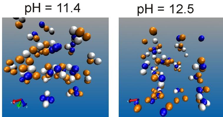
**Figure 2:** Snapshot of the formed aggregates in suspensions of PbO, Nb<sub>2</sub>O<sub>5</sub> and MHC particles at pH 11.4 (left), and 12.5 (right). PbO – orange, Nb<sub>2</sub>O<sub>5</sub> – white, MHC – blue.
