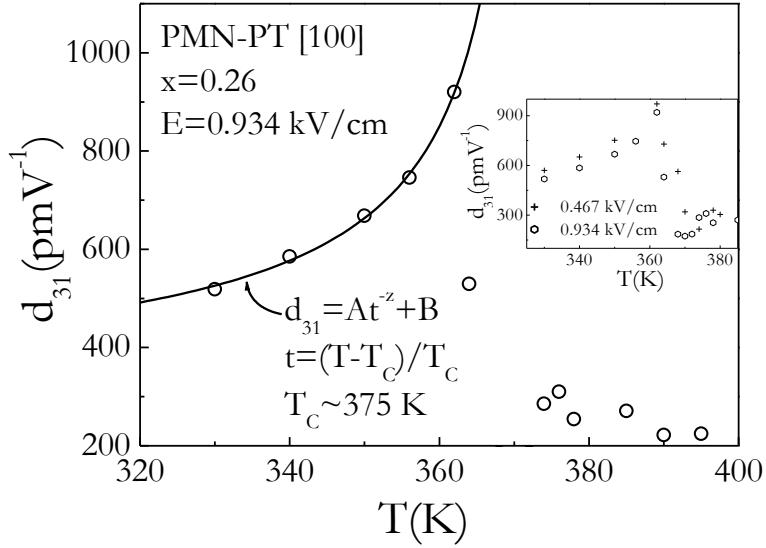
**Figure 2:** Solid line represents a fit to the power law ansatz of temperature dependent piezoelectric coefficient at  $E=0.934$  kV/cm. The inset shows temperature dependence of the  $d_{31}$  at  $E=0.467$  kV/cm and  $0.934$  kV/cm.
