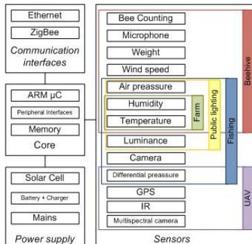
**Figure 2:** VSN Modularity as used in testbeds
