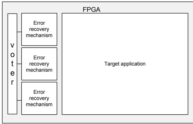
**Figure 4:** Self-reparable system with internal error recovery mechanism in TMR
