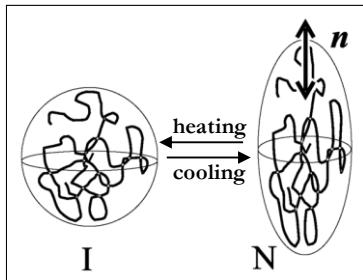
**Figure 1:** LCEs spontaneously stretch/shrink due to the temperature changes.
