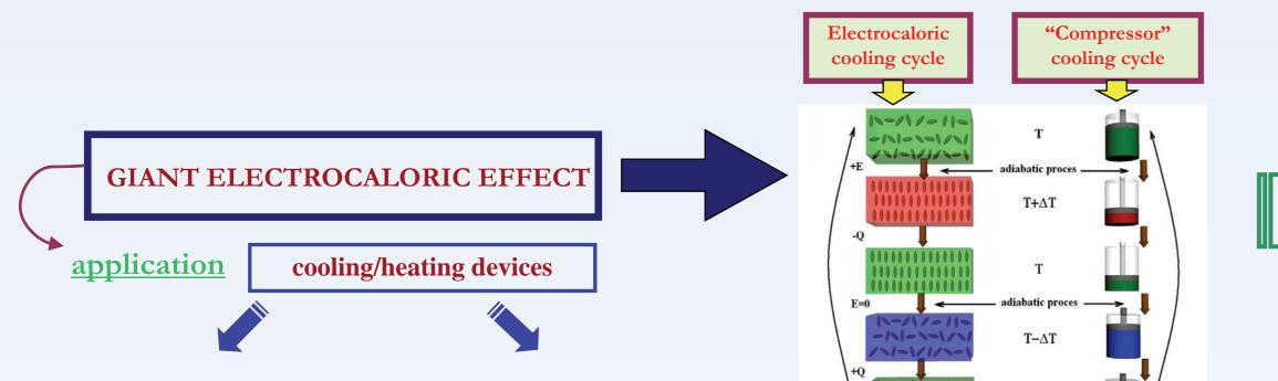
Electrocaloric cooling cycle is comparable with a corresponding cooling cycle of a classic compressor where pressure p of the gas is changing.
